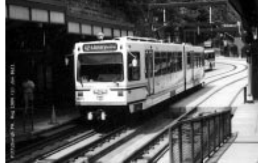
Light rail does not require a fully separated right-of-way because power is supplied by overhead catenary, rather than an electrified rail. It can operate on rights-of-way, which are fully or partially separated or at street level alongside traffic, as shown in these photographs from Baltimore (left) and Pittsburgh (right).
