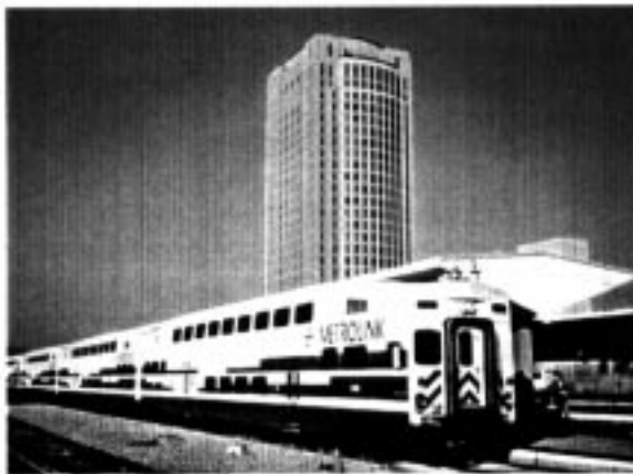
Commuter rail service between suburban or rural locations and central cities can be provided either by a locomotive pulling or pushing single- or bi-level passenger coaches (left) or by self-propelled diesel or electric rail cars (right).
