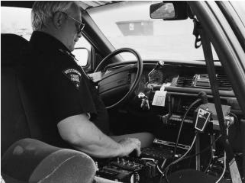
A Wisconsin state trooper accesses driver information on a mobile data computer. The computers, installed in all State Patrol vehicles, are linked directly to state and national driver and crime information databases – keeping the airwaves clear for emergency calls from dispatchers. (Department of Transportation)
